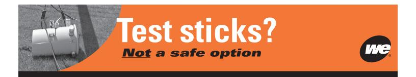
"Test sticks" are not a safe method to determine if a downed power line is energized. All downed power lines should be considered energized until an electric utility employee verifies and grounds the line.
