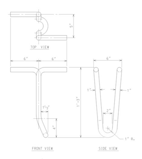
NOTE: MATERIAL, 1" ROUND STEEL, THOROUGHLY GALVANIZE AFTER BENDING. DEVELOPED LENGTH -  $40^{1}/2$ ".
