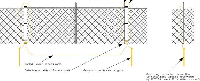
180.50.10) Fence Ground Interconnected With Station Ground Grid
