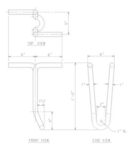
NOTE: MATERIAL, 1" ROUND STEEL, THOROUGHLY GALVANIZE AFTER BENDING. DEVELOPED LENGTH - 40<sup>1</sup>/<sub>2</sub>".
