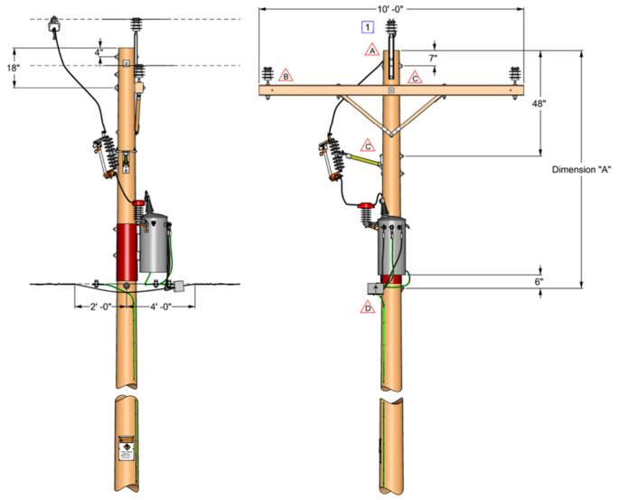
1 Maximum line angle on pin insulator shall be limited to 5 degrees.
