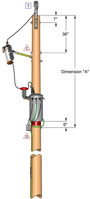
1 Maximum line angle on pin insulator shall be limited to 5 degrees.
