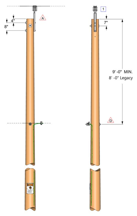
1 Maximum line angle on pin insulator shall be limited to 5 degrees.
