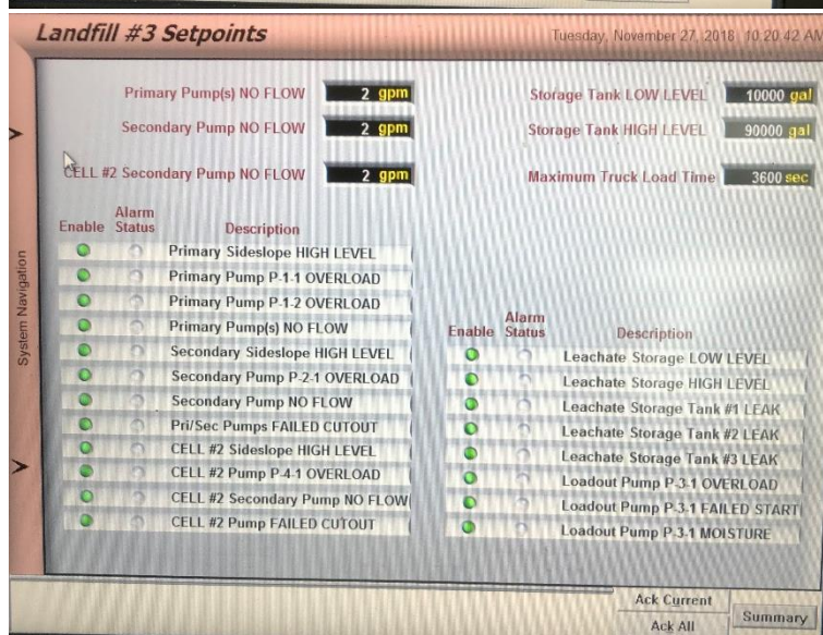
Photo 13 – Landfill No. 3 leachate collection system controls screens.
