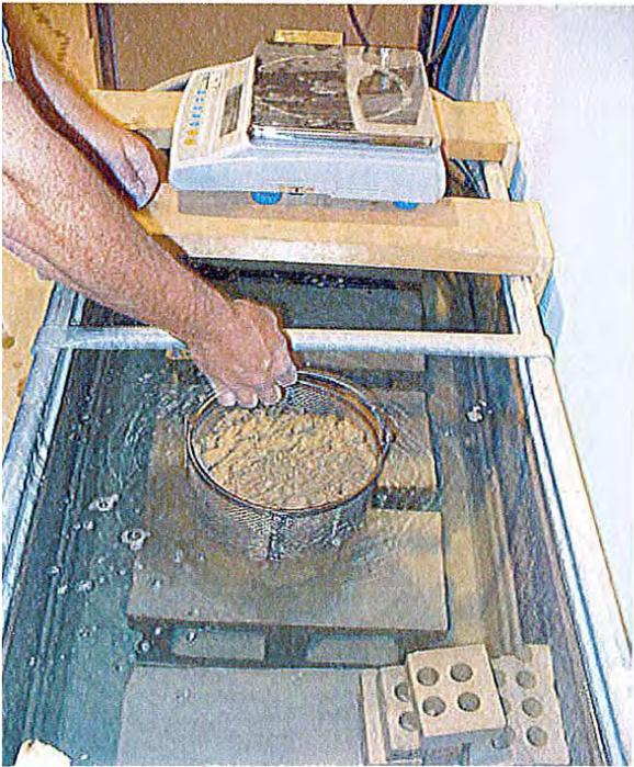
Upper left photograph shows the soaking of the aggregate for obtaining the weight in the saturated surface dry condition. Upper right photograph shows the drying of the aggregates to saturated surface dry condition. Lower left photograph shows the basket and balance used to obtain the underwater weight of the sample for determination of the aggregate's specific gravity.
