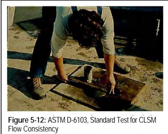
Figure 5-12: ASTM D-6103, Standard Test for CLSM Flow Consistency
