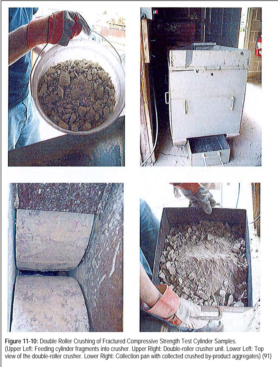
Figure 11-10: Double Roller Crushing of Fractured Compressive Strength Test Cylinder Samples. (Upper Left: Feeding cylinder fragments into crusher. Upper Right: Double-roller crusher unit. Lower Left: Top view of the double-roller crusher. Lower Right: Collection pan with collected crushed by-product aggregates) (91)
