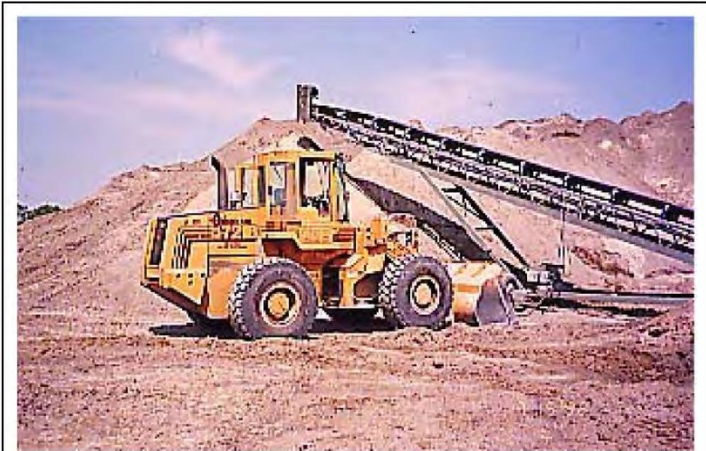
Figure 6-9: Coal ash recovery from the Pleasant Prairie Power Plant ash landfill for use as granular base course material
