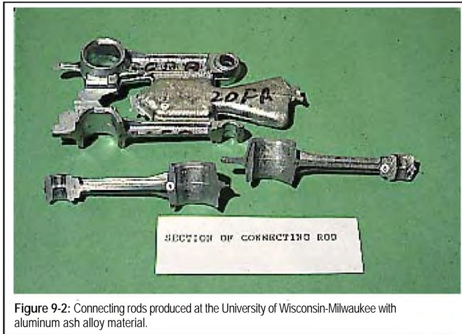
Figure 9-2: Connecting rods produced at the University of Wisconsin-Milwaukee with aluminum ash alloy material.
