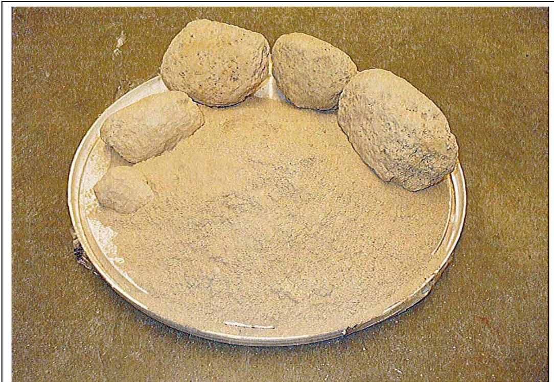
Figure 11-9: LA Abrasion Equipment Crushing of CLSM Test Cylinder Samples after Strength Testing (91)
