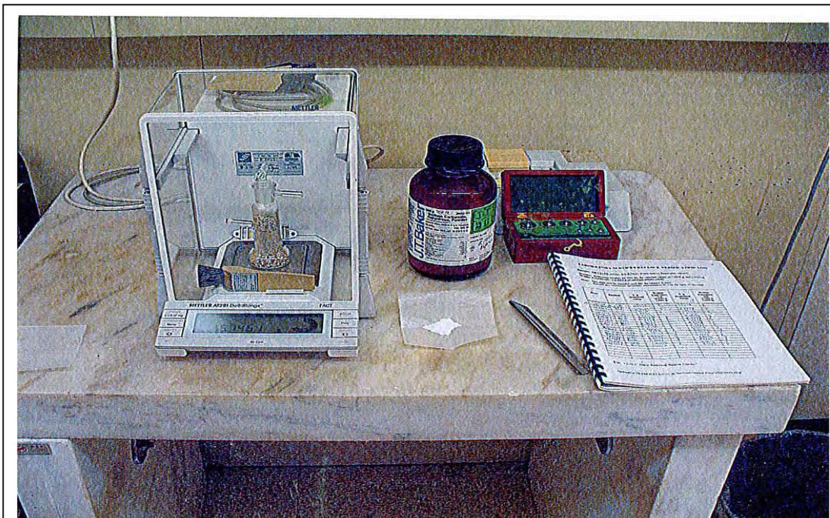
Figure 11-4: Balance, Calibration Weights, Ascarite Absorber and Standard Sample (Reagent Grade  $\text{Na}_2\text{CO}_3$ ) (91)
