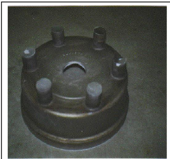
**Figure 9-1:** Brake drum cast with aluminum ash alloy material in Manitowoc, Wisconsin
