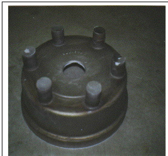
Figure 8-1: Brake drum cast with aluminum ash alloy material in Manitowoc, Wisconsin
