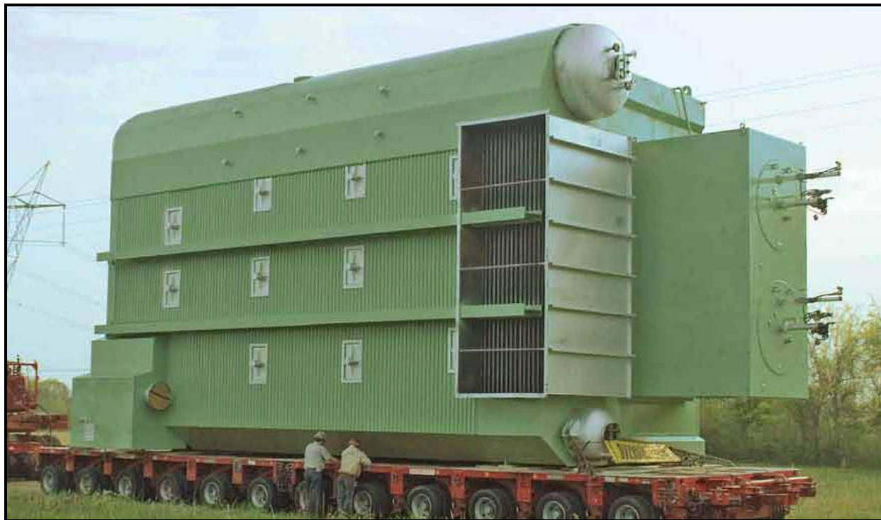
FIGURE 1-1. Large FM type water tube package boiler (The Babcock & Wilcox Company).
